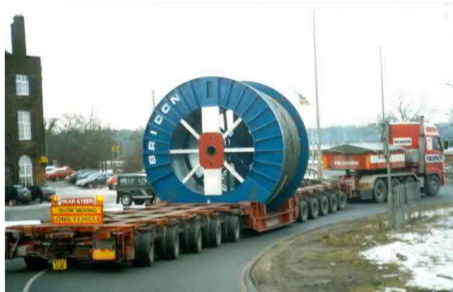
Plate 1. Transport configuration for a cable reel off approximate 100te
